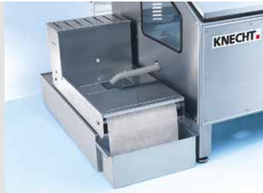
Belt filter coolant unit
